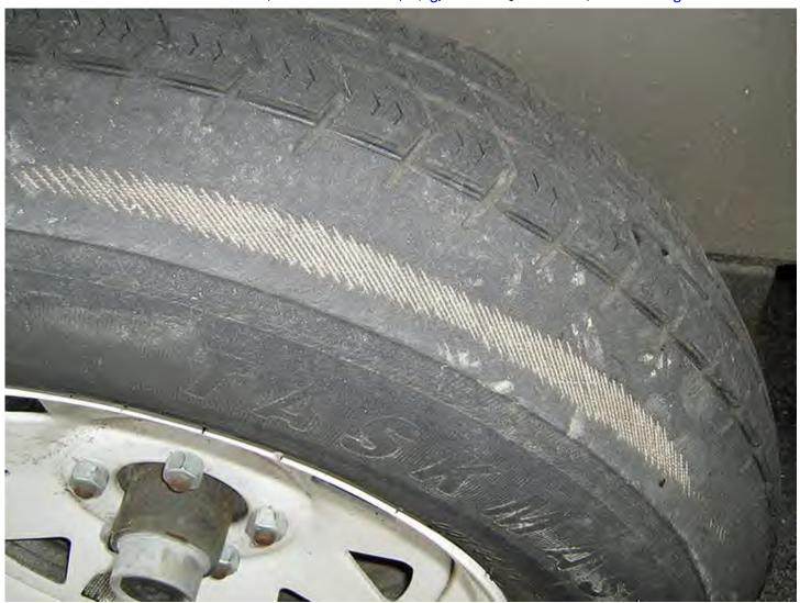
Finally, anytime after installing a new suspension lift or adding new steering and suspension components, you should get a front end alignment. Make sure you use a company who knows how to deal with 4x4 vehicles and won't sell you on simply getting a four-wheel alignment, as you do not have independent rear suspension in your Jeep. A good alignment shop will also know how to properly set your vehicle's caster and toe angle.
