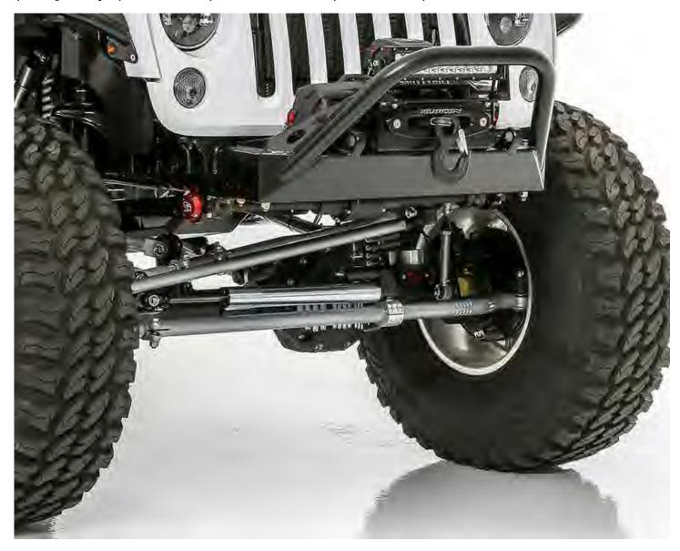
Your Jeep's tie rod and tie rod ends should be next on the hit list. To check these, use a jack to lift up the front of the Jeep and then have a friend grab one wheel and twist it back and forth. If the tie rod doesn't move, but the ends seem to wiggle, then they most likely need replacement. Of course, if the rubber boot is torn or damaged that is another replacement sign. Plus, if the actual tie rod is bent then definitely look at swapping out that <u>tie rod</u>
