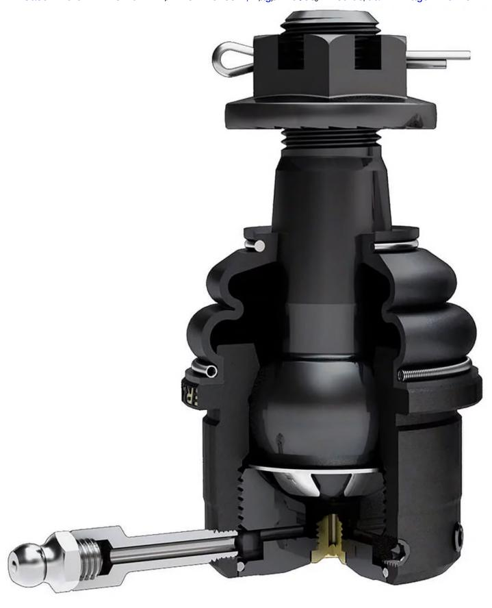
The vehicle's ball joints are yet another important part to investigate when trying to eliminate death wobble. These ball joints connect the steering knuckle to the axle, are encased in rubber boots filled with grease and designed to help smooth out steering. If these boots are damaged and grease is
