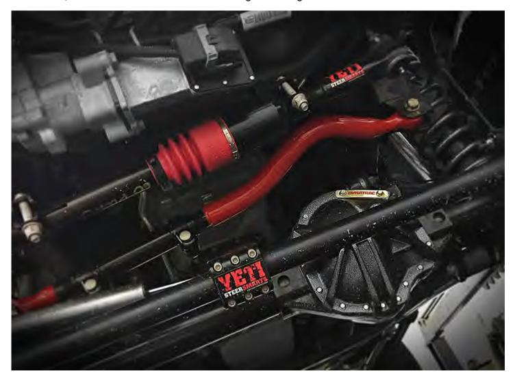
After tightening all bolts, the first part to attack is your factory track bar. This is a product designed to absorb a lot of force and keep your vehicle's axle from drifting side to side. Over time though, this force can deform the bar's frame side bolt hole, causing the bolt to become loose and track bar bushings to wear out. The result can be a significant amount of play in the track bar.
