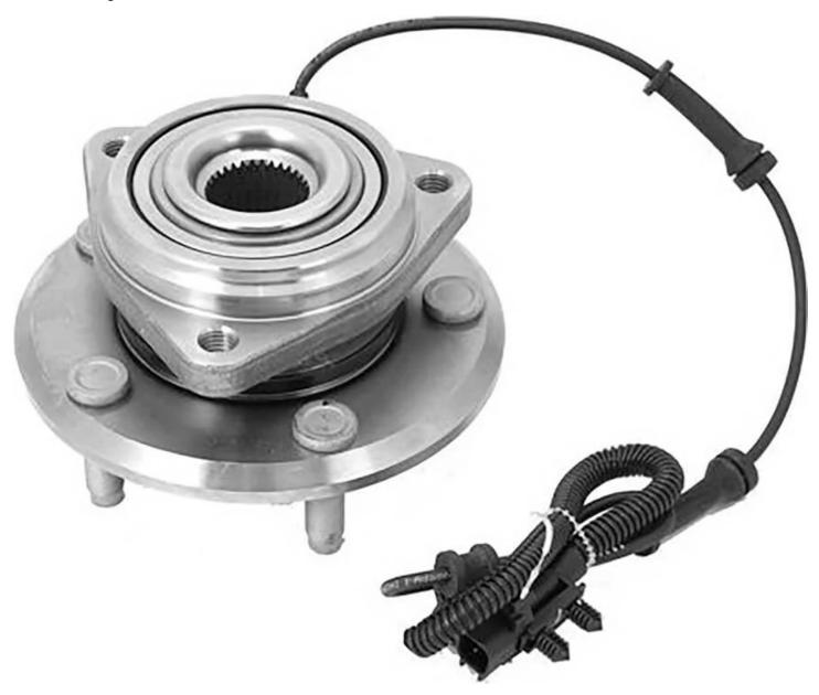
Worn wheel bearings may contribute to death wobble as well and are very easy to test. Jack up one of your Jeep's front wheels and grasp the tire at the 12- and 6-o'clock position, then wiggle the tire. If you feel movement, then you most likely have a worn wheel bearing. Check the other side as well.
